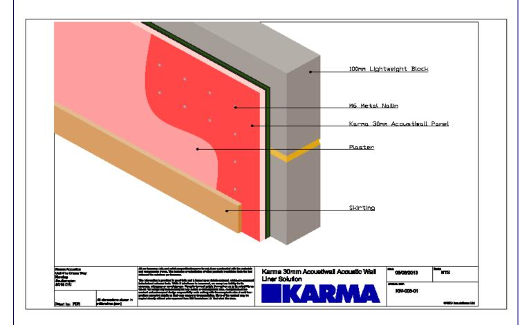
Direct to masonry wall solution (30mm Thickness As Above) with M6 x 65mm Metal Nailins to new/existing block/brick walls.
