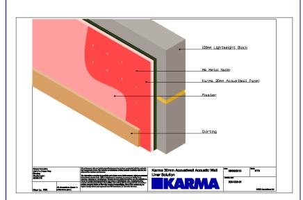
**Application:** Easy to fit, slimline solution for new/existing masonry walls where the original walls are to be converted into party or separating walls between dwellings
